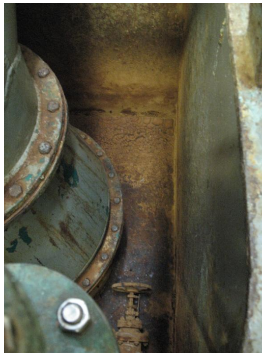
Figure 18: Bow thruster sea bay suction well
