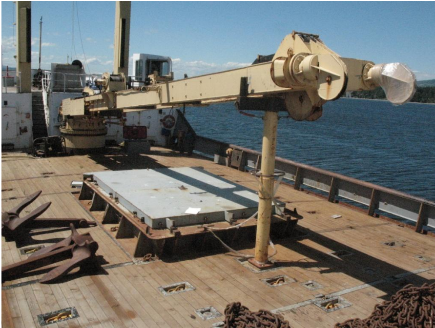
Figure 9: Buoy Derrick, main hatch, well deck, and anchors
