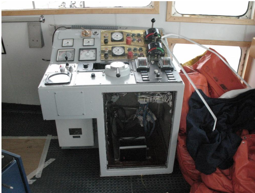
Figure 25: Stbd bridge wing maneuvering console
