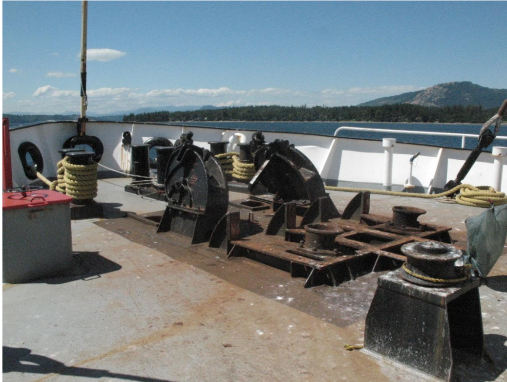
Figure 11: Windlass bedplate, chain stoppers, fairleads on foc'sle
